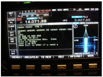
There are 8 RTTY and 8 PSK transmit memories which can be easily edited using an USB keyboard. Transmitting from these memory locations can be performed with or without an attached USB keyboard.
