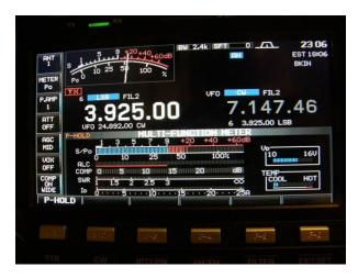
Note the many choices for the meter display which looks and operates like a mechanical meter.
