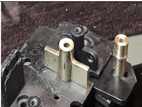
Ultimate Transmitter Company, 1930s mini bug rebuild. Cracked pot metal parts replaced by new machined brass...
