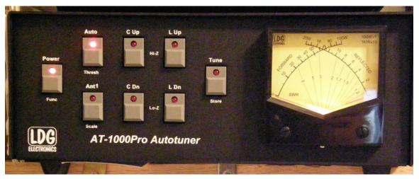
Picture below is of my old AT-1000 after tuning a 2.5:1 SWR showing about 40 watts of output from my ICOM 756 PRO II.
