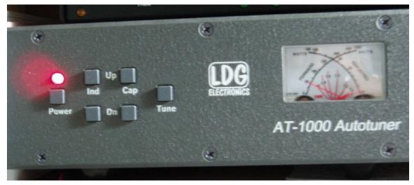
Below is a picture of the AT-1000Pro meter after tuning a 2:5:1 SWR showing about 40 watts from my ICOM 756 PRO II.
