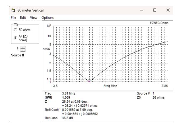
Note that this SWR curve is too narrow for both phone and CW simultaneously.
